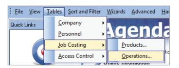
Next, create each required operation. Remember that the code defined against the operation is the code that must be selected when entering data at the shop floor data collection terminal.
