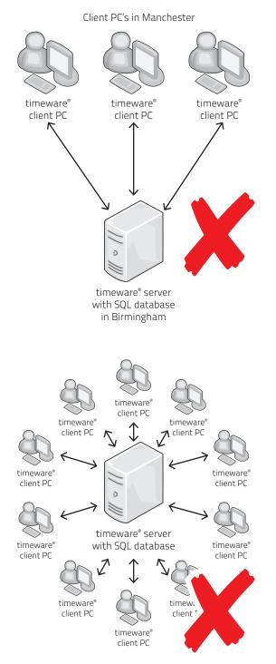
In this example we have client PC's that are located in Manchester and a timeware® server in Birmingham. This setup would cause a massive amount of problems with connectivity that would result in an unusable system. It is NOT recommended to have the client PC's connecting over long distances. Instead, it is recommended to have the client and server be on the same local network.
